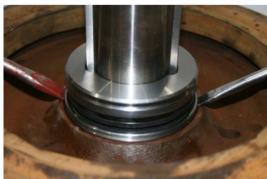
Fig. 10: Prising out the mechanical seal using pry bars
