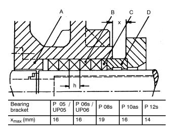
Fig. 2 Uncooled arrangement
