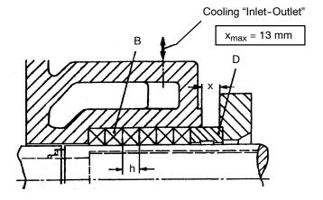
Fig. 3 Cooled arrangement Bearing bracket P 02a, P 03, P 04, UP02, UP03, UP04
