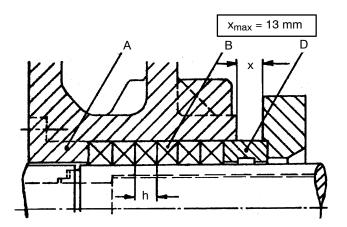
Fig. 1 Uncooled arrangement Bearing bracket P 02a, P 03, P 04, UP02, UP03, UP04
