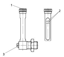
Fig. 2: Oil level gauge
