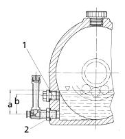
Fig. 1: Fitted oil level gauge
