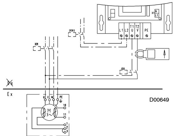
Fig. 15: Measuring the heating current
