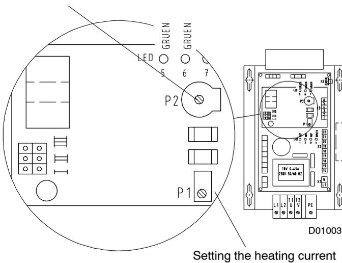
Fig. 13: Adjusting the heating current, MHG 35/220-500
