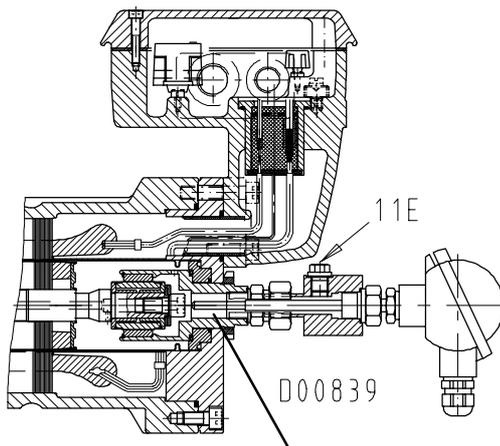
Temperature sensor in rotor space
