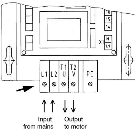
Fig. 4: Connecting the power components
