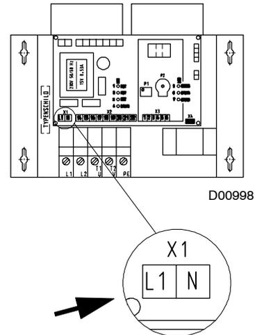
Fig. 6: Connecting control components MHG 100/220-500
