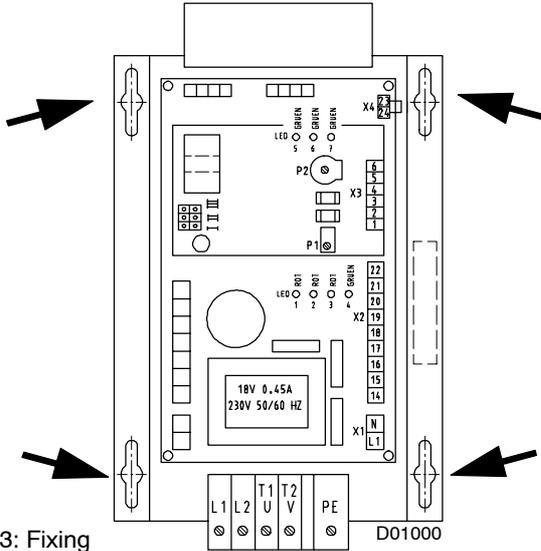
Fig. 3: Fixing
