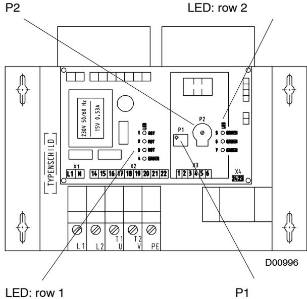
Fig. 10: Potentiometers and LEDs MHG 100/220-500
