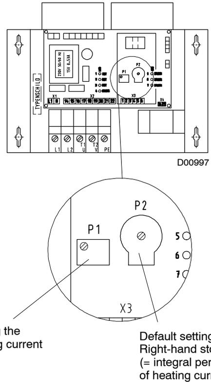
Fig. 14: Adjusting the heating current, MHG 100/220-500
