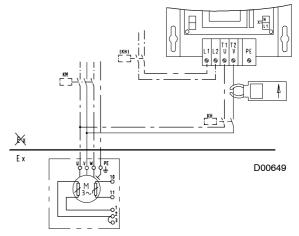
Fig. 15: Measuring the heating current
