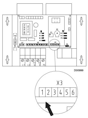
Fig. 8: Heater ON/OFF MHG 100/220-500
