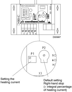
Fig. 14: Adjusting the heating current, MHG 100/220-500
