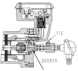
Temperature sensor in rotor space
