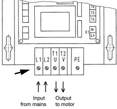
Fig. 4: Connecting the power components
