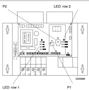
Fig. 10: Potentiometers and LEDs MHG 100/220-500
