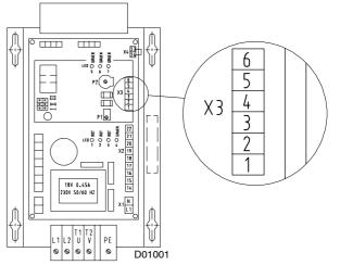
Fig. 7: Heater ON/OFF MHG 35/220-500, MHG 35/220-500KS, MHG 35/220-500MS
