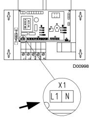
Fig. 6: Connecting control components MHG 100/220-500
