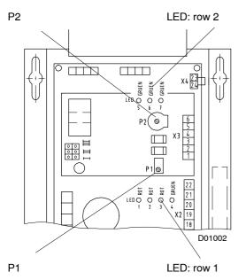
Fig. 9: Potentiometers and LEDs MHG 35/220-500, MHG 35/220-500KS, MHG 35/220-500MS
