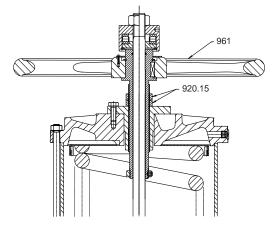
Figure 21: Fail-close actuator (LAP-SF)
