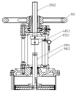
Figure 16 - Double-acting actuator (LAP-AZ)
