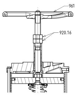
Figure 20: Fail-open actuator (LAP-OF)
