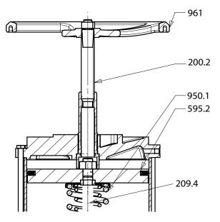
Figure 17: Fail-open actuator (LAP-OF)
